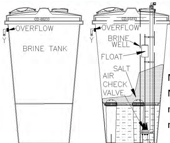
Brine tank c/w internal safety float and brine grid. For units up to and including 450,000 (15 ft 3 ) brine line is also included. For all larger units, brine line is not supplied and is normally piped in 3/4" or 1" pvc.
