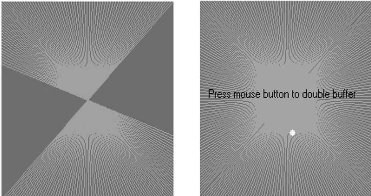
**Figure 27-2** Output from **DoubleBuffer** without (left) and with (right) double buffering
