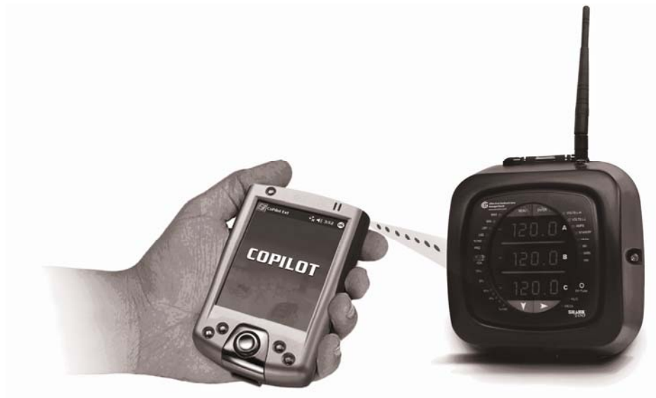
Figure 5.1: Communication with IrDA Port
