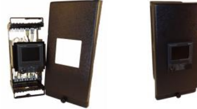
Schneider/SUSI ION7400 retrofit in large Basler case
