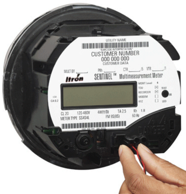
Figure 2.4 Connecting the Battery
