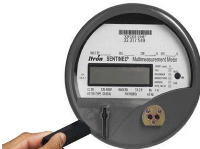
Figure 3.4 Activating the Magnetic Switch
