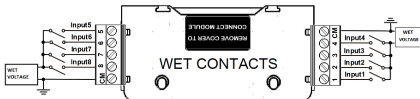
Figure 2-22 8 DI - Digital Input Connection – Wet contact model
