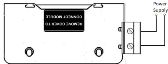
Figure 2-26: AUX_PS Module Connection
