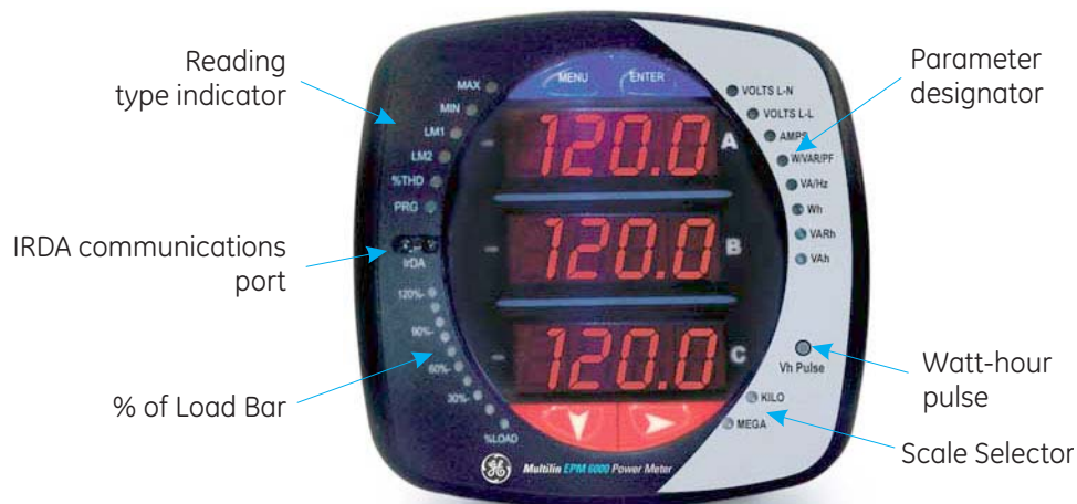
Figure 6-1: Faceplate of EPM 6000 Meter with Elements
