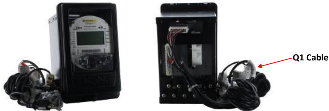
Front and rear view of SWIWS9-EL-M8650 in FT-21 Elite case with Q1 cable installed
