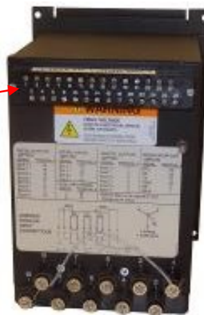
JEMS24I Module connects to back of JEMSTAR case
