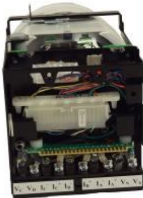
Transdata Module (TM1) connects to back of Transdata case
