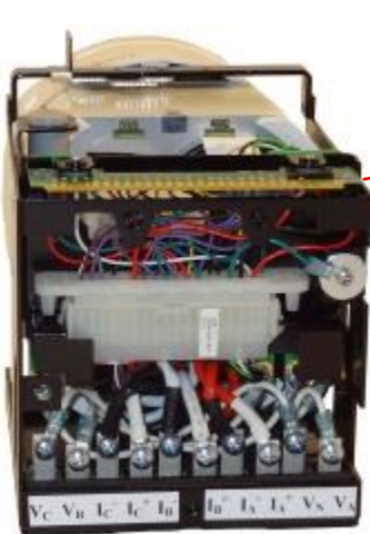
JEMSSC Module connects to back of JEMSTAR case
