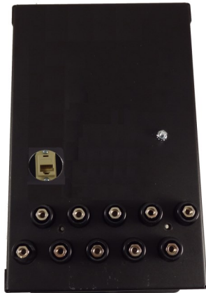
Front and rear view of ION 8650 retrofit in Westinghouse/ABB case with Ethernet
