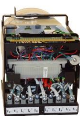
JEMX Module connects to back of JEM10 case
