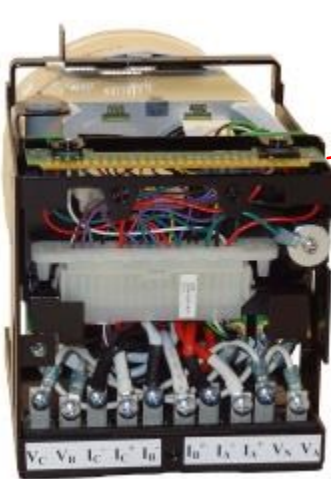
JEMS4 Module connects to back of JEMSTAR case
