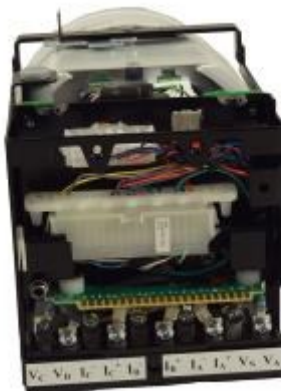
Transdata Module (TM3) connects to back of Transdata case
