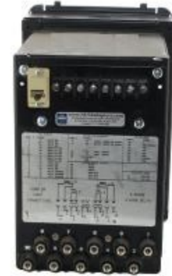
Rear View of JEMSTAR/JEM10 small case with BP Module installed
