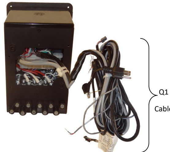
Rear View of ES, EPM 5100 and kV meter in S1 case with ION 8650 and Q1 Cable
