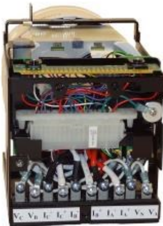
JEMSXP Module connects to back of JEMSTAR case
