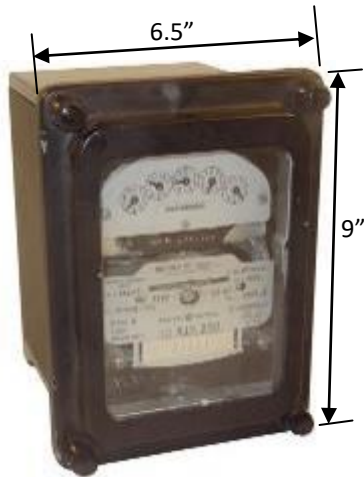
Front and rear view of GE DS-63 meter in S1 Case
