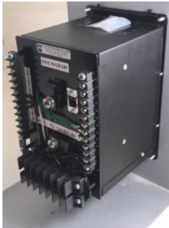
Rear view of SWCWSIIJEM9 ION 8650 in FT-21 case
