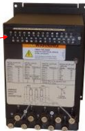
JEMS2 Module connects to back of JEMSTAR case
