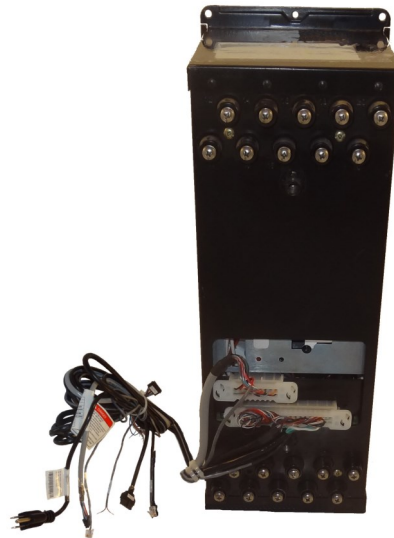
Rear View of FT-31 case with Q1 Cables
