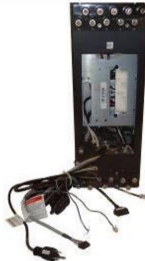
Rear View of JEM1 Tall Case with Q1 Cable (Original FT-21 Cable) (Schneider #C0H6C7B & C0H6C7C)
