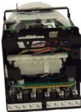
Transdata Module (TM5) connects to back of Transdata case
