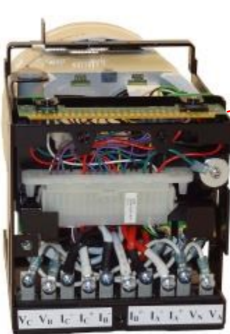
JEMS2 Module connects to back of JEMSTAR case
