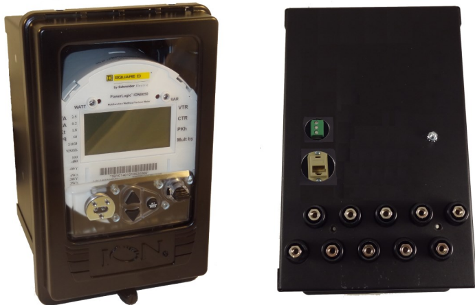
Front and rear view of ION 8650 retrofit in Westinghouse/ABB case with Ethernet and AUX
