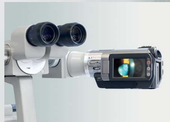
DigiCam system with commercial camera
