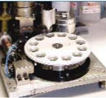
Lenses secured by highly precise automated adhesive dispensers
