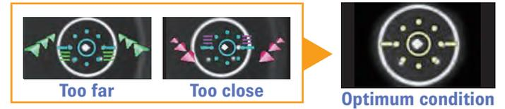
**Supine Position Mode** When tilting the instrument 60° or more downward, the supine position mode automatically starts. When measuring from the patient's side, the cylinder axis is compensated by 90°, and is displayed.
