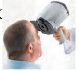
**Removable Magnetic Occluders** Removable magnetic occluders cover unmeasured eye to enable the measured eye to fixate on the target.
