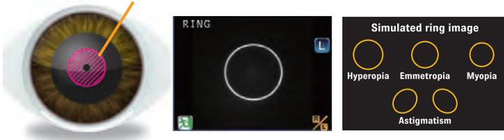
**SynchroScan Technology** The HandyRef-K uses "SynchroScan Technology": Measurements start when alignment is achieved, and data is captured when alignment becomes optimal. This provides a more stable, effective, and efficient measurement.
