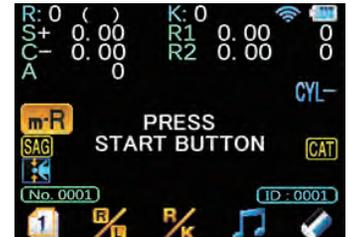
**Axis Correction Function** An internal sensor detects the inclination of the instrument to display the automatically corrected axis.\*
