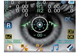
**Focusing Indicator** By detecting the distance between the instrument and the patient's eye, the alignment guide mark is displayed on the screen to facilitate smooth measurement.
