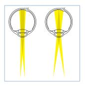
Unique to the BQ 900, an optional stereo variator reduces the 13° angle to 4.5°. Thus, an enlarged binocular field of view is possible even with myopia or through small pupils. This also aids the observation, without additional lenses, of the peripheral fundus and vitreous. It improves fundus viewing for imaging applications.
