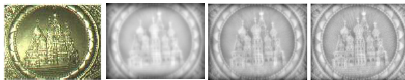
Figure 2.10: Result of the resolution-enhanced algorithm. The first image is the acquired frame, the second is the depth field retrieved from the first; the successive ones are the depth maps retrieved with the enhancing at different levels (2x and 4x)
