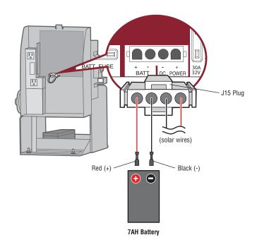
To use a 33AH battery in place of the 7AH battery, follow the instructions below. The 33AH application requires the 33AH wire harness (Model K94-37236).
