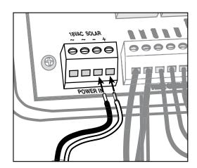
Insert one transformer wire into an **18VAC** terminal. Insert the other transformer wire into the remaining **18VAC** terminal (*see illustration*). Transformer wires can be connected to the **18VAC** terminals regardless of color.
