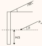
active thurst act at a height H/3 from the base of the wall and at an angle equal to backfill inclination.
