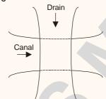
Drain taken ove the canel in a super passage(line plane of crossing)
