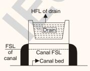
Typical cross-section of a super passage.
