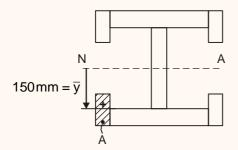
Shear force in nail at  $P = \frac{VA\overline{y}}{I} \times pitch$
