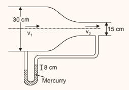
When the water flows, the differential manometer shows a deflection of 8cm of mercury (Hg). The values of specific gravity of mercury and water are 13.6 and 1.0, respectively. Consider the acceleration due to gravity,  $g = 9.81 \text{ m/s}^2$ . Assuming frictionless flow, the flow rate (in  $m^3/s$ , round off to 3 decimal places) through the duct is \_\_\_\_\_.
