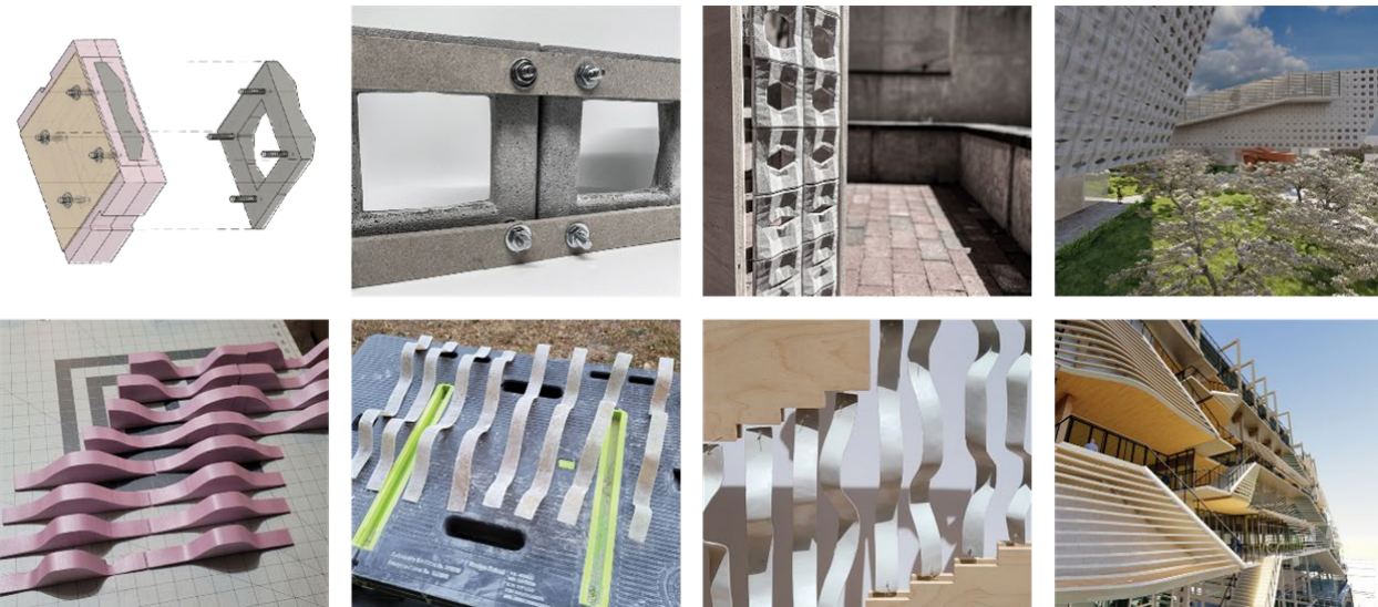
Fig. 6 The images on the top row show a student project that focused on 2-part CNC milled formwork to create custom tiles with variable opening sizes to control daylighting. The aperture sizes were informed by computational analysis of daylighting. The bottom row of images shows a project that utilized robotic hot wire cut foam as a mold for fiberglass louvers.
