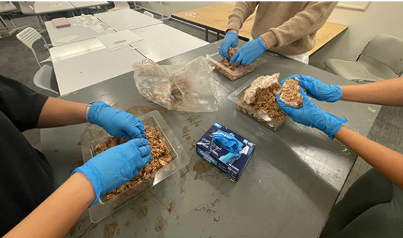
Fig. 4 Regrinding and packing forms with mycelium and hemp mixture. Student Work.
