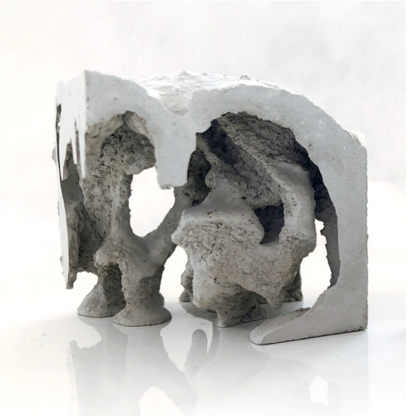
Fig. 9 Rockite casting with water soluble biodegradable biofoam L. Locke, 2019
