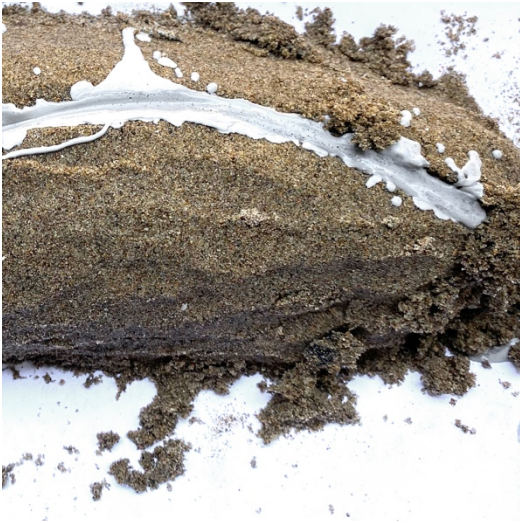
Fig. 12 Rockite casting with damp sand formwork, T. Tran, 2022
