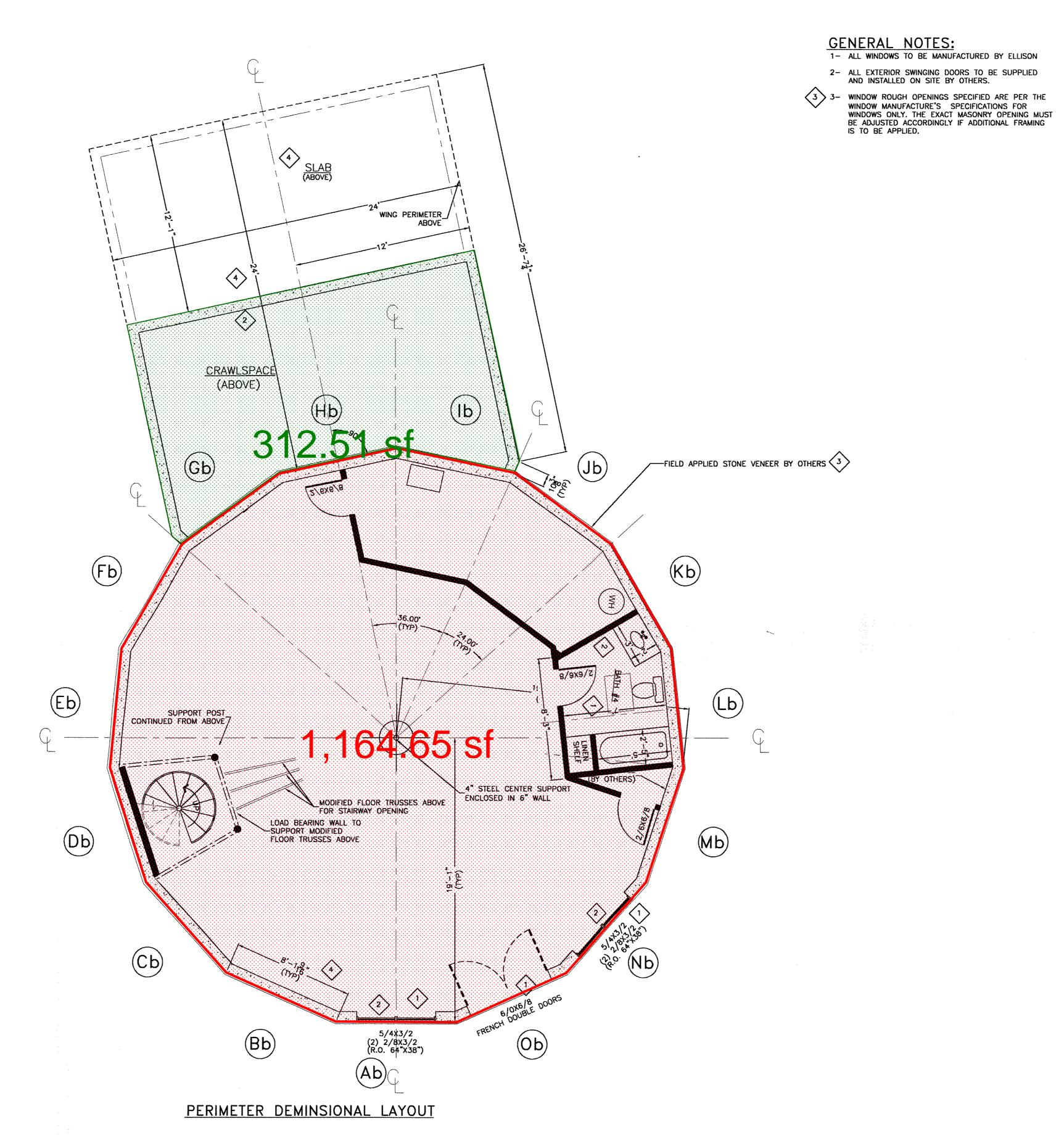
ADDED BATH. ADDED WINDOWS OP PANELS AND AND DED F.DBL DOOR OPANEL ON. ADDED SPIRAL STAIRS WITH SURROUNDING WALLS. ALL AS PER CUSTOMERS MARKED PRINT.
