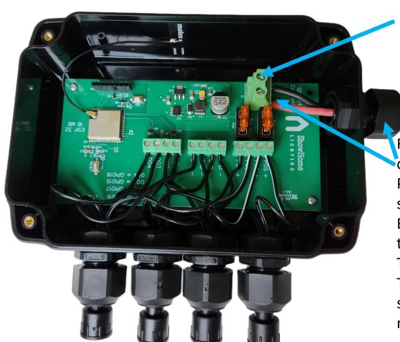
Back the screws out before inserting wires
