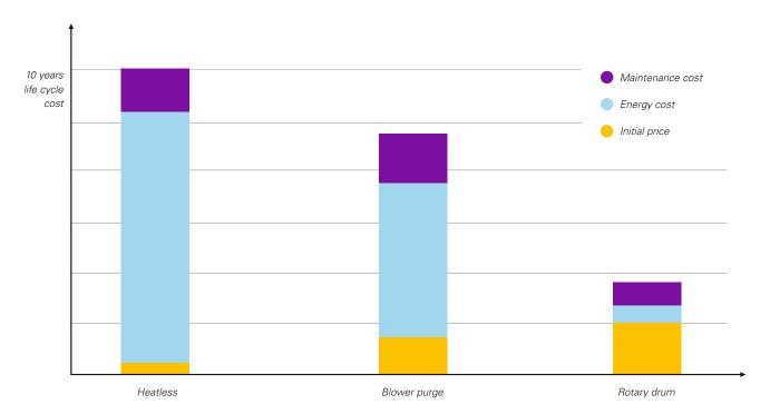
The heatless desiccant dryer is the most expensive to operate as 15-20% of its rated flow capacity is consumed as purge air. The rotary drum dryer can lead to significant energy savings because of its unique design and controls. Even compared to a blower purge dryer, rotary drum dryers can save up to 50% of the lifecycle cost.
