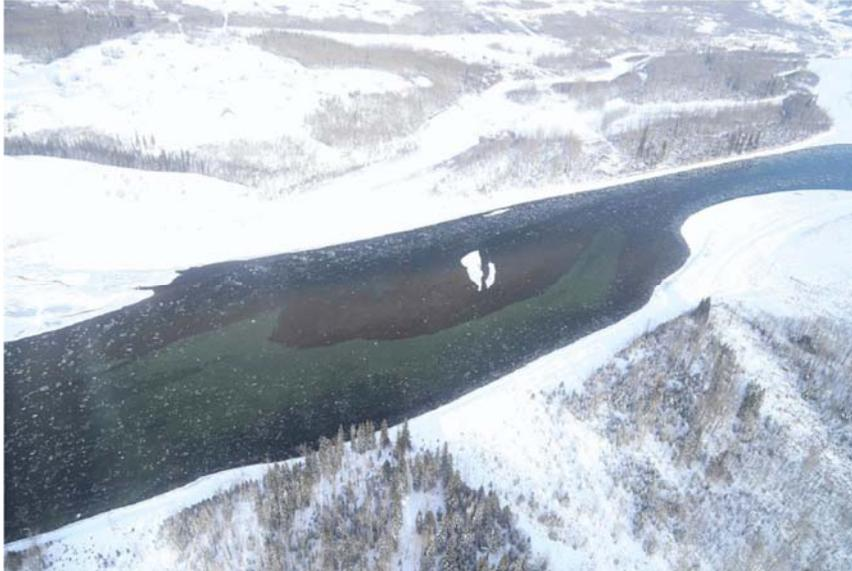
**Figure 5.10** Anchor ice observed on the Peace River, Alberta. Flow is from left to right and the river width is ~300m. (*Photo courtesy of M. Jasek.*)
