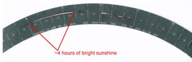
**Figure 9.1** Prior to 1996, sunshine balls were used to obtain manual measurements of hours of bright sunshine at Canadian meteorological stations. A glass ball (top photo) would focus the sunlight which, when sufficiently strong, would burn a hole in the replaceable card (bottom photo) providing an indication of the number of hours of bright sunshine. This could then be converted to an estimate of incoming solar radiation based on location and date.
