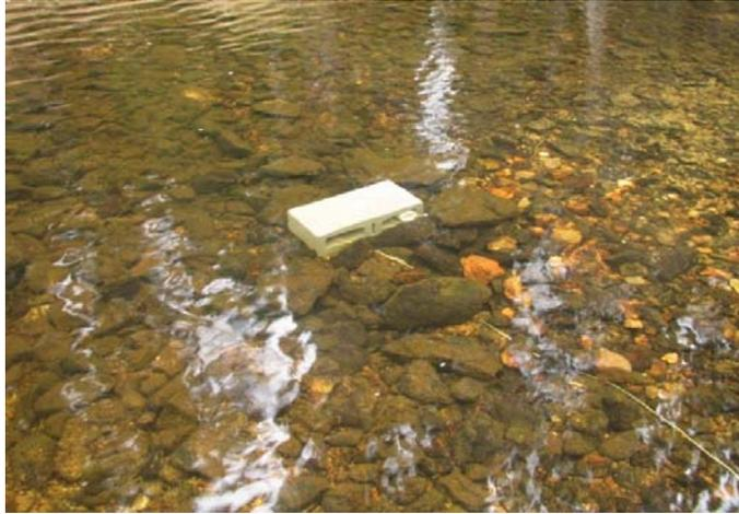
**Figure 9.9** Water temperature sensor installed on a small creek. Here, the sensor has been attached to a concrete block, for ballast, and tethered to the bank with a coated steel cable. (*Photo courtesy of J. Nafziger.*)
