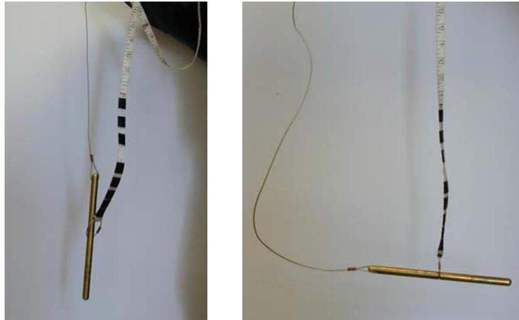
**Figure 9.15** Simple ice thickness measurement apparatus. (Photos by F. Hicks)
