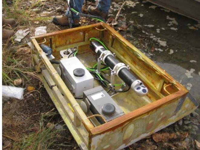
**Figure 9.12** Example setup for deployment of shallow water ice profiling sonars for surface ice measurement. (Photo courtesy of T. Ghobrial.)
