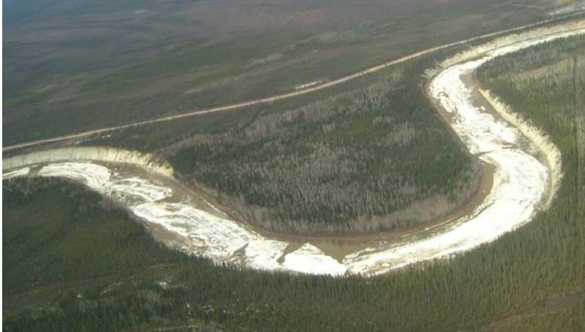
**Figure 3.13** Sheet ice accumulation on the Hay River, NWT. Flow is from left to right. (Photo by F. Hicks.)
