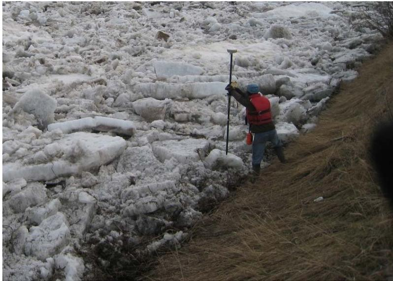
**Figure 9.18** Measuring the top-of-ice profile along a river ice jam.
