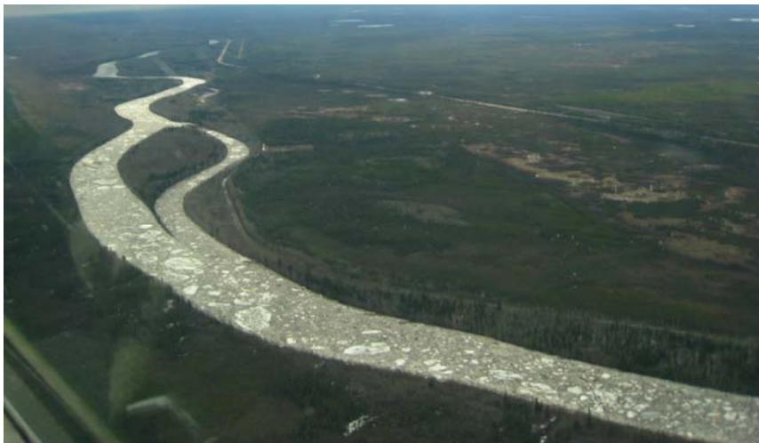
**Figure 3.15** Ice accumulation (ice jam) on the Hay River, NWT. Flow is from top to bottom. *(Photo by F. Hicks.)*
