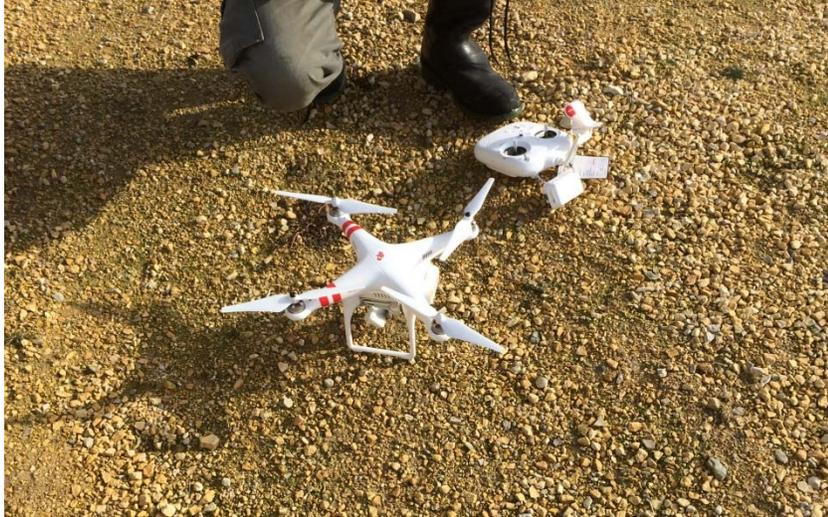
**Figure 9.14** Example of a small drone aircraft used for photographing surface ice conditions. *(Photo courtesy of A. Wall and S Clark.)*
