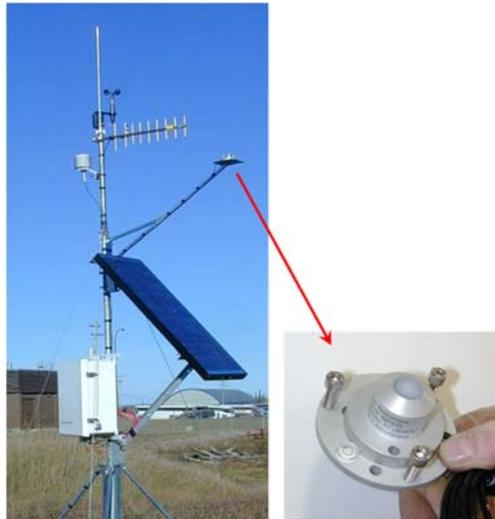
**Figure 9.2** A pyranometer can be used to obtain automated measurements of incoming solar radiation. (*Photos by F. Hicks.*)
