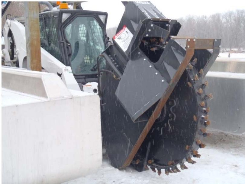
**Figure 8.4** Ice cutting machine used to ‘score’ the ice cover on the Red River, Manitoba. (*Photo courtesy of S. Clark.*)
