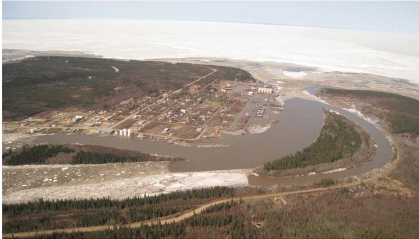
**Figure 3.16** Ice jammed against the intact ice on Great Slave Lake, NWT. Note the flooding along the left bank of the Hay River. Flow is from left to right.
