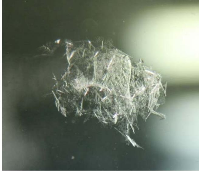
**Figure 2.5** Frazil floc observed in the laboratory.
