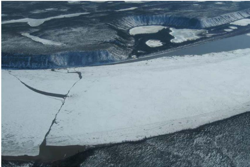
**Figure 3.10** Transverse crack observed on the Mackenzie River, NWT.
