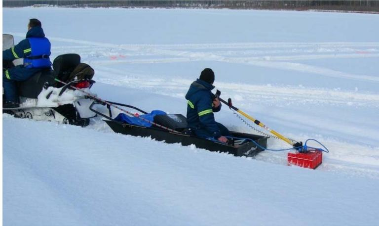
**Figure 9.16** Example application of a GPR device being towed behind a snowmobile. (Photo source: F. Hicks)
