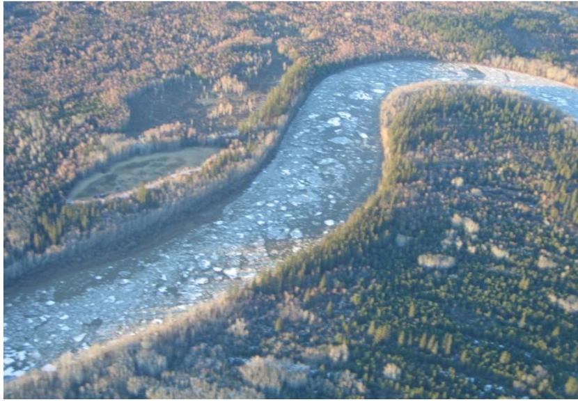
**Figure 3.17** Ice run following ice jam release event on the Athabasca River in Alberta. Flow is from left to right – notice the ice jam reforming further downstream (top right corner of the photo). (Photo by F. Hicks.)
