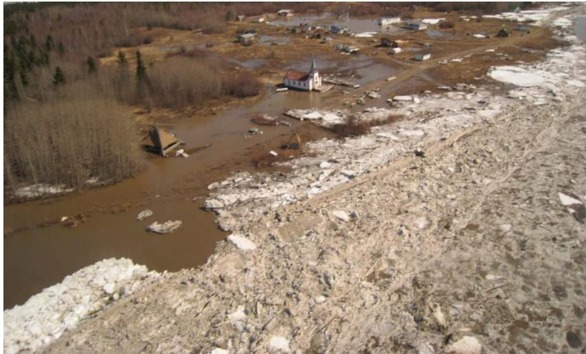
**Figure 1.1** Ice jam flood during 2008 breakup on the Hay River, NWT. This photo was taken looking upstream along the ice jam and shows the flooding in the adjacent old village of the Kátl'odeeche First Nation. (*Photo by F. Hicks.*)
