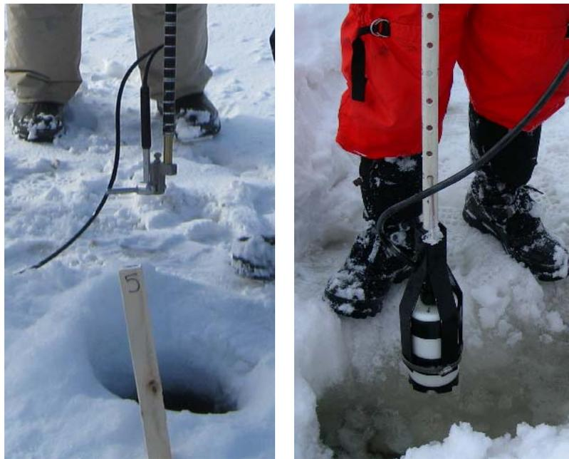
**Figure 9.5** *Left:* Acoustic Doppler Velocity (ADV) current meter used for measuring flow velocity at a discrete point. *Right:* Acoustic Doppler Current
