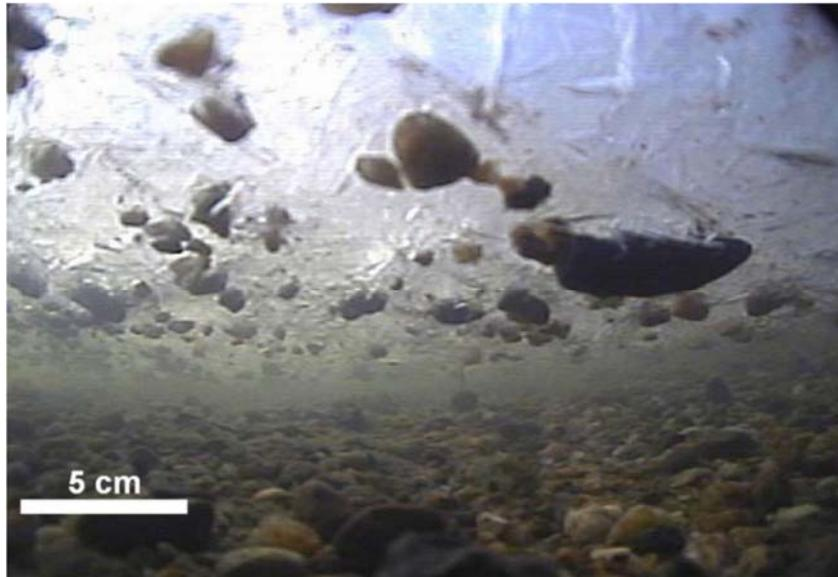
**Figure 2.22** Sediment rafting by anchor ice.
