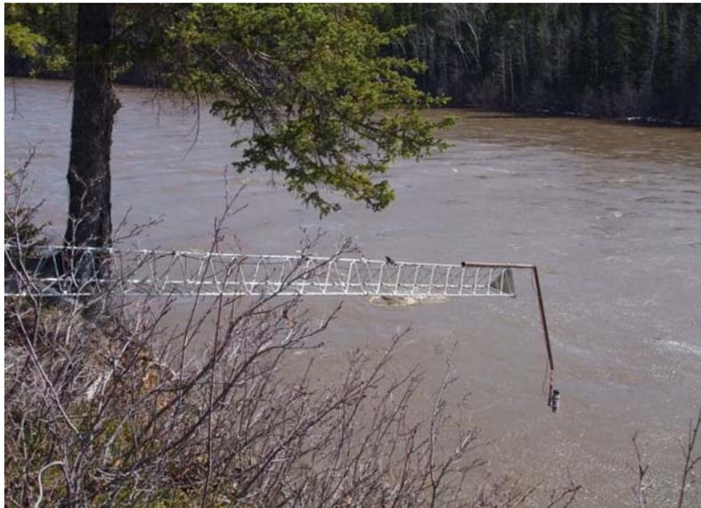
**Figure 9.4** Acoustic water level sensor mounted on a boom and suspended over a river. (Photo courtesy of J. Nafziger.)
