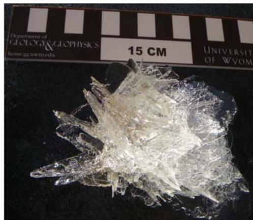
**Figure 2.16** Large anchor ice crystals from the Laramie River in Wyoming. (Photo courtesy of E. Kempema.)
