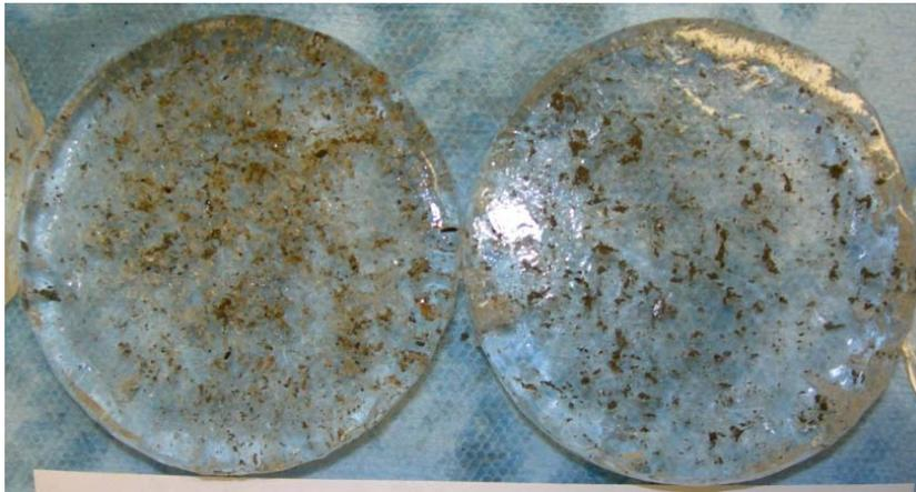
**Figure 4.5** Example of organic and inorganic impurities seen in horizontal slices through frazil ice from the Athabasca River in Alberta. Samples are 7 cm in diameter.
