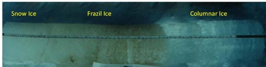
**Figure 2.31** Ice core sample from the Mackenzie River, illustrating the various ice components typically found within a river ice cover. (Photo source: F. Hicks.)
