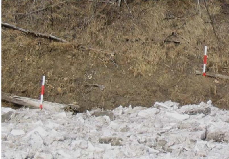
**Figure 9.19** Staff gauges may be used for measuring top-of-ice levels in areas that are inaccessible during ice jam events. (*Photo by F. Hicks.*)
