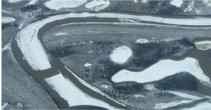
**Figure 3.11** Here the shorefast ice has melted away and the remaining ice has broken into discrete sheets; however the ice sheets cannot maneuver around the bends and so the ice is not yet moving.
