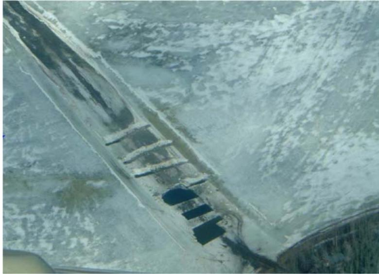
**Figure 8.9** Aerial view of the Athabasca River, Alberta site shown in Figure 8.8. The low albedo of the open water areas created help to accelerate the ice deterioration as the water absorbs short wave radiation and then melts the ice from the underside. (*Photo courtesy of Alberta Environment and Sustainable Resource Development.*)
