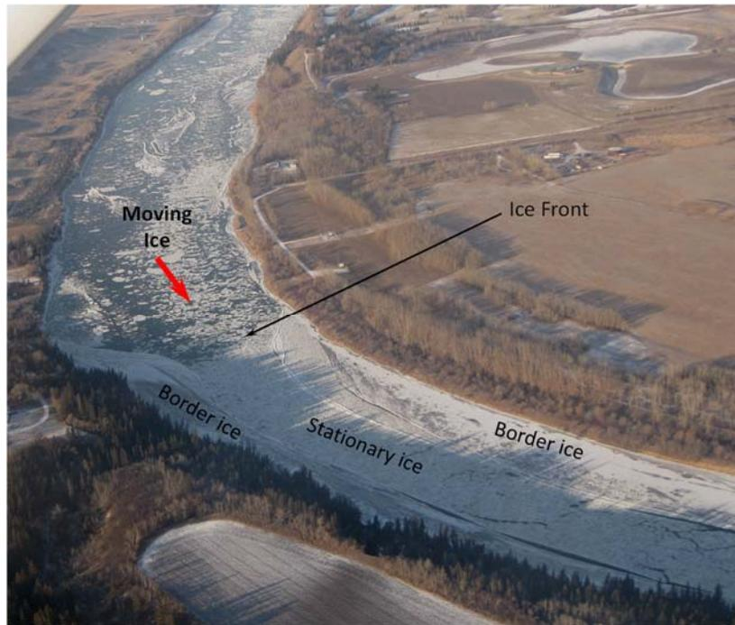
**Figure 2.25** Natural constrictions, and those enhanced by border ice encroachment, present likely spots for bridging to occur.
