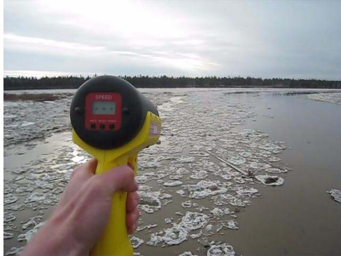
**Figure 9.7** Specially adapted radar guns can be used to measure the velocity of floating ice pans and moving ice floes. (*Photo source: F. Hicks.*)
