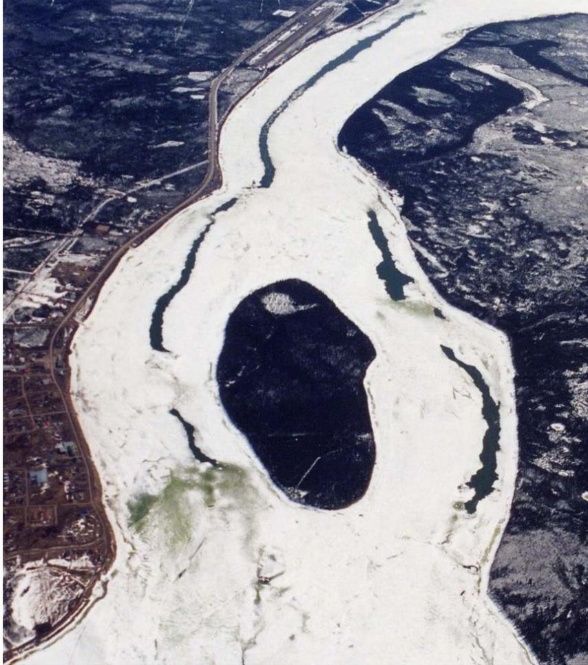
**Figure 3.6** Overflow from open leads on the Mackenzie River, NWT. This is a sign of rapidly rising water levels. (*Photo by F. Hicks.*)
