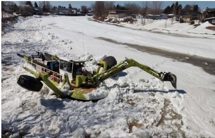
**Figure 8.6** Mechanical equipment used to break up the ice cover on the Sainte-Anne River in Québec. The machine, known as an Amphibex, uses its bucket to pull itself onto unbroken ice and its self-weight will cause the ice to break. *(Photo courtesy of T. Simard-Robitaille.)*
