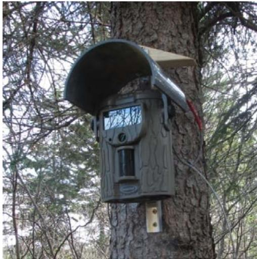
**Figure 9.10** Game camera installed on tree for ice process documentation.
