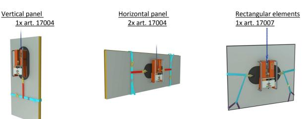
The falling safety devices are executed by means of lifting straps with hooks, which must be hooked to the suction pad. During use the following must take place.
