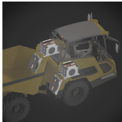
Lithium Ion Batteries
