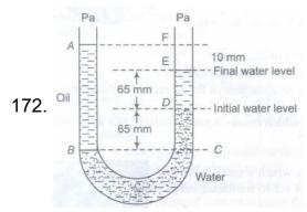
A U tube with both ends open to the atmosphere, is partially filled with water and oil, which is immiscible with water, is poured into one side until it stands at a distance of 10 mm above the water level on the other side. Meanwhile the water rises by 65 mm from its original level (see diagram). The density of the oil is
