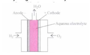
(*i*) In the given cell, hydrogen and oxygen are bubbled through porous electrodes
