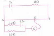
Q392.Calculate the voltmeter reading and the amount of current passing through a circuit.
