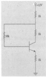
Q446.In the circuit shown in the figure, the BJT has a current gain ( $\beta$ ) of 50. For an emitter-base voltage  $V_{EB}$  = 600 mV, calculate the emitter-collector voltage  $V_{EC}$  (in volts).
