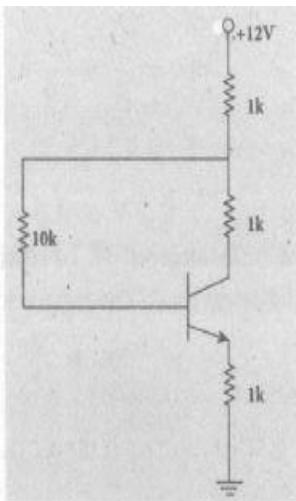
Q446. In the circuit shown in the figure, the BJT has a current gain ( $\beta$ ) of 50. For an emitter-base voltage  $V_{EB} = 600$  mV, calculate the emitter-collector voltage  $V_{EC}$  (in volts).
