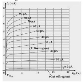
Q449. The current gain of a common emitter transistor circuit shown in figure is 120. Draw the DC load line and mark the Q point on it. ( $V_{BE}$  to be ignored).
