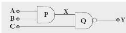
Q337.In the combination of the following gates, write the Boolean equation for output Y in terms of inputs A and B.
