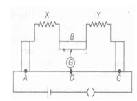
The figure shows experimental set up of a meter bridge. When the two unknown resistances X and Yare inserted, the null point D is obtained 40 cm from the end A.
