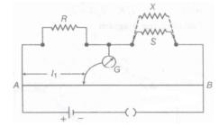
(i) In the circuit diagram given below AB is a uniform wire of resistance  $15\Omega$  and length 1m is connected to a cell  $E_1$  of emf 2V and negligible internal resistance and a resistance R.
