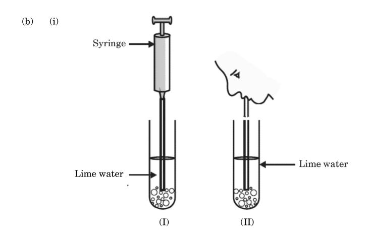
In the experimental set-up shown above in diagram (I) atmospheric air is being passed into lime water with a syringe while in diagram (II) air is being exhaled into lime water. The time taken for the lime water to turn milky in both the test tubes is different. Give reason.
