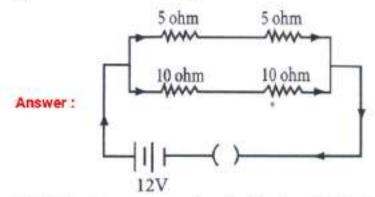
(i) The 5 Ω resistors are connected in series. Therefore, their effective resistance = (5 + 5) = 10 Ω
