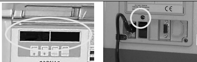
Fig. III-7 – On stand-by the electronics unit display is off, while the cp1 connection module LED indicator stays on.
