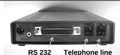
Fig. IV-5 : Detail of the metal detector connectors
