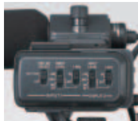
XLR 2-ch Audio Input Adaptor (Select Switch)
