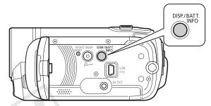
While the camcorder is on, hold DISP. pressed down for more than 2 seconds.
