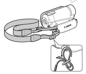
Pass the ends of the shoulder strap through the strap mount on the grip belt and adjust the length of the strap. You can also remove the grip belt and attach the shoulder strap directly to the rear bracket on the camcorder.
