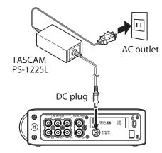
A hook (cord holder) to fix the cord of the AC adaptor is on the right side panel. Wrap the cord around the hook when connecting it to prevent it from being disconnected during use.
