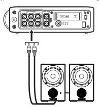
Powered monitor speakers or amplifier and speakers
