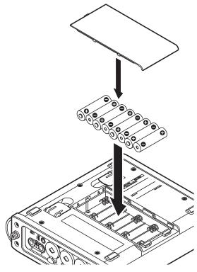
When using AA batteries, set the battery type so that the unit can accurately display the remaining battery charge and determine the necessary minimum remaining charge for operation. (See "Setting the battery type" on page 46.)
