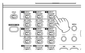
LINE: Set the switch to LINE when the line output jack of an external device is connected to the analog input on this unit.
