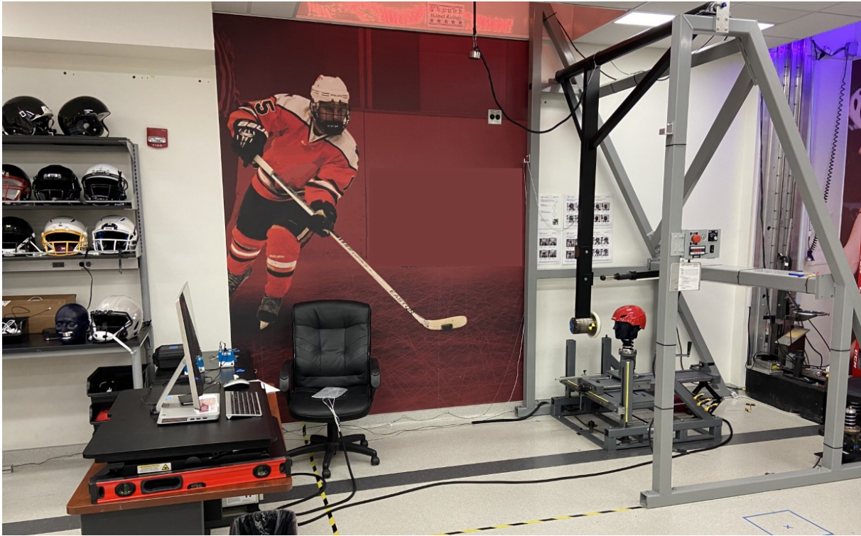
Figure 2: The front impact condition is shown on the right with the pendulum system.
