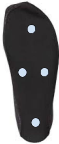
Fig 3.3 Diagram of Force Sensor Positions on Sock
