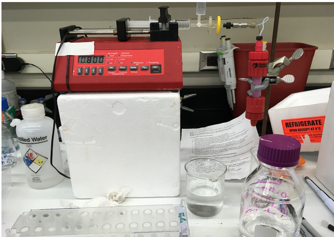
IMAC purification equipment (mechanical loading tool): currently set to 0.8 mL/min
