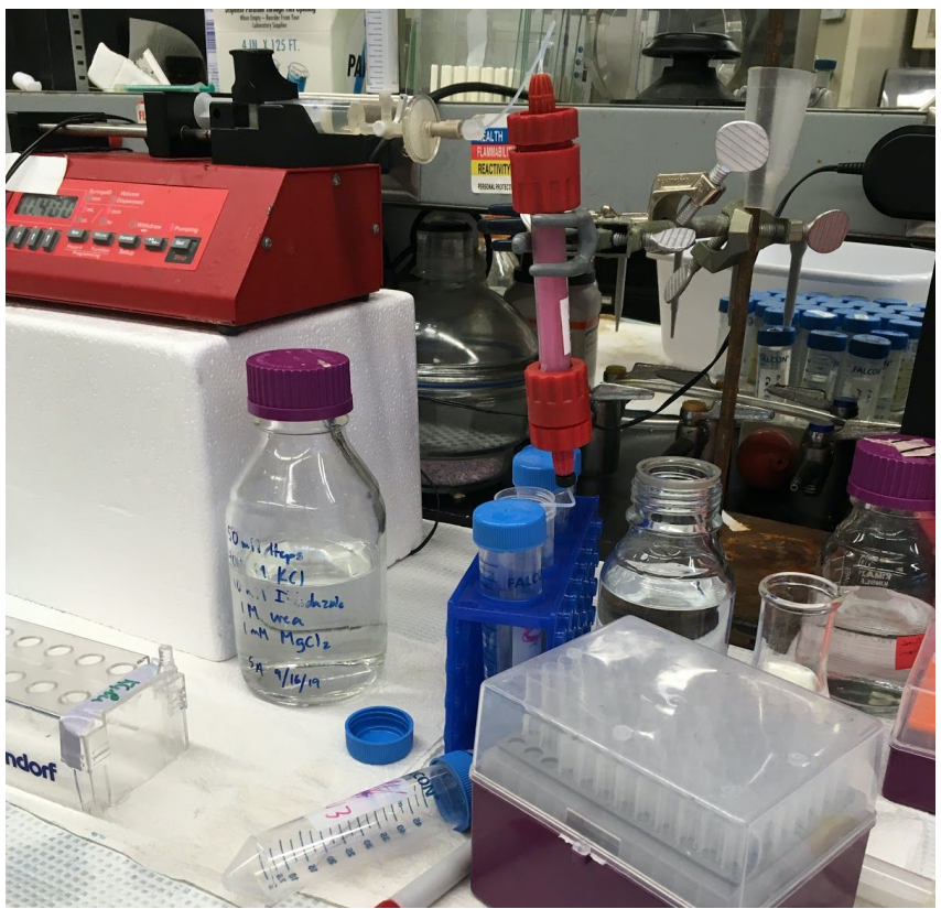
Left: IMAC purification (collecting final protein fractions)
