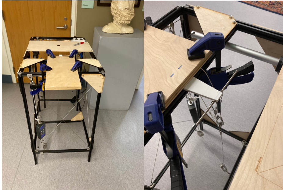
Figures 3 & 4: The school's weight table that was used for testing and the mount with a wing in it
