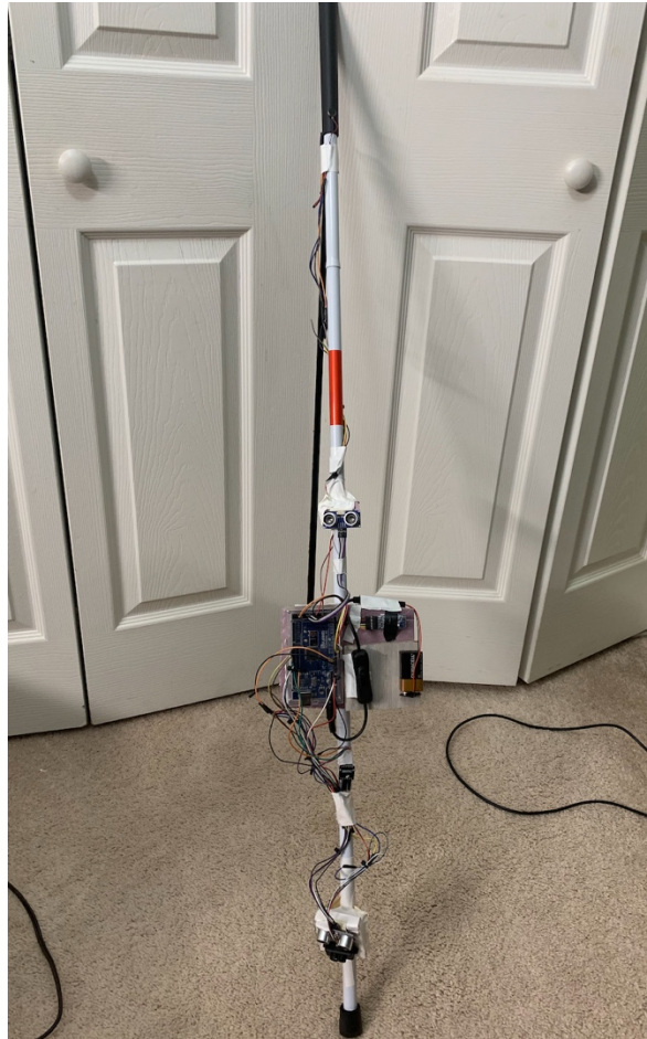
Figure 7: Front side view of the final product with all sensors, modules, and Arduino board fitted to respective angles and locations
