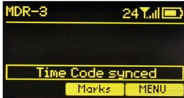
B. MDR3 time code accuracy and stability. The MDR3 real-time clock is tuned at the factory to better than 1 ppm accuracy at ambient temperature of 20C. To maintain 1 frame accuracy at 24fps or 30 fps, the MDR3 should be jammed at 8 hour intervals or less, at ambient 20C.
