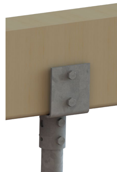
Typical Connection Detail
