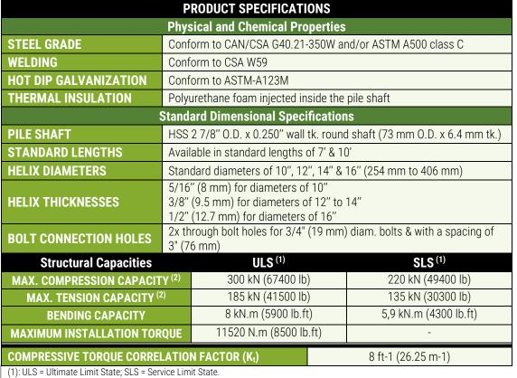
(2): The specified capacities are only applicable to the steel assembly where the pile shaft is laterally supported. In all cases, the mechanical capacity of the extension must be validated by a licensed engineer, and with considerations for column buckling if installed in liquifying soils, peats or bogs
