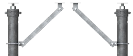
Typical connection detail – "K" bracing
