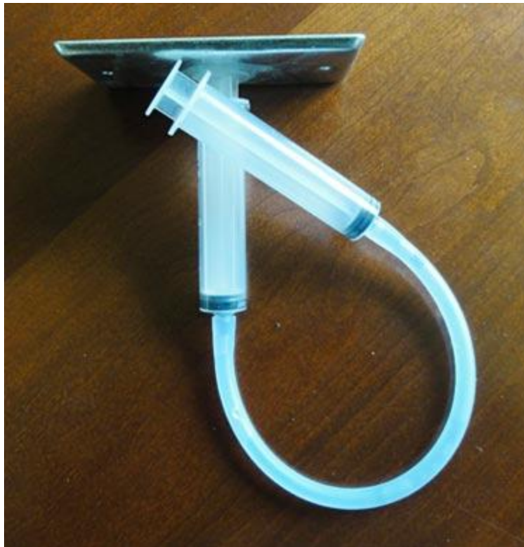
Figure 6. This image shows the master syringe attached to a slave syringe and its metal plate.
