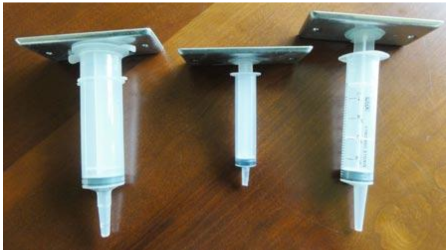
Figure 5. This image shows the three slave syringes and wall plates used in the experiment. Each slave syringe/metal plate pair comprises half of a model hydraulic lift.
