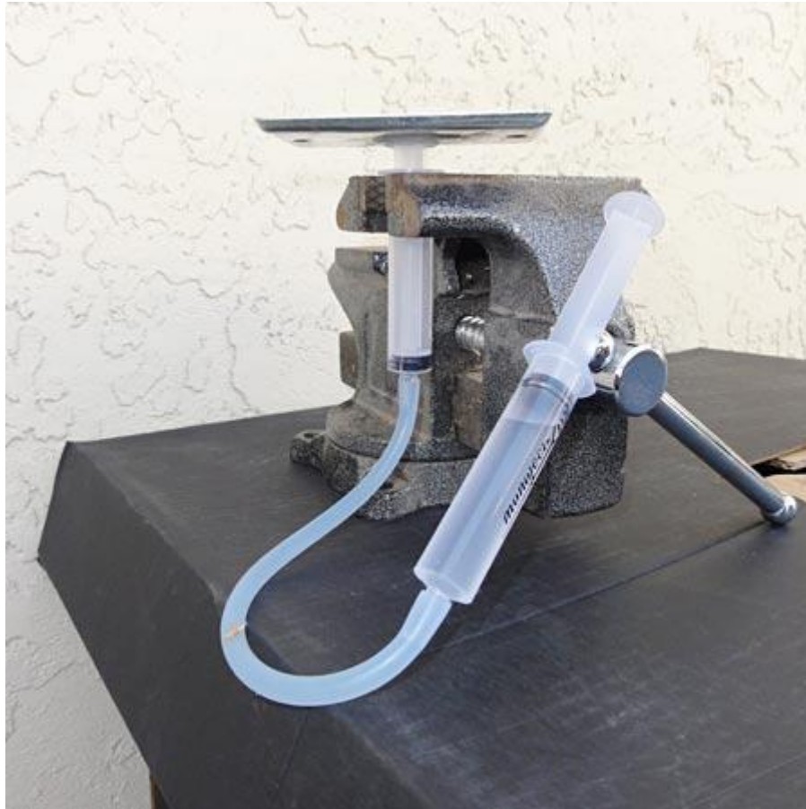
Figure 7. Here is a completed 12 cc model hydraulic lift, where the lift is properly held and supported by the vise.
