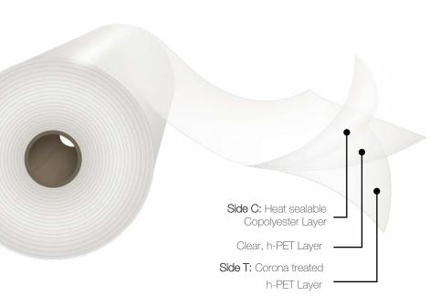
Consider EC-TC only as an inverted reel (heat sealable copolyester inside and corona treated outside), properties and applications remain the same.
