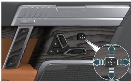
The lumbar support can be adjusted up, down, forward and backward by the adjustment button.
