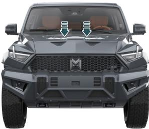
1. Press down the engine hood until the locking latch touches the locking mechanism;
