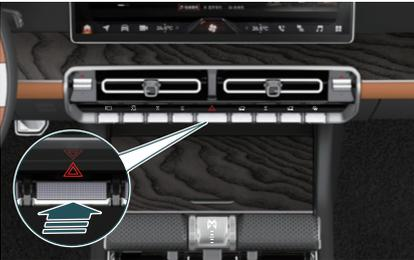
The hazard warning lamp switch is located in the middle of the instrument panel control panel.
