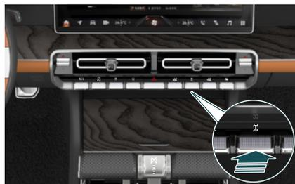
Press the CrabWalk mode button to turn the CrabWalk function on/off. When activating the function, the vehicle needs to be stationary and the steering wheel needs to be returned to the center position.
