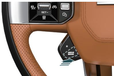
Press the highway mode button on the steering wheel to switch to highway mode: Standard mode → Sports mode → Comfort mode → INDIV.
