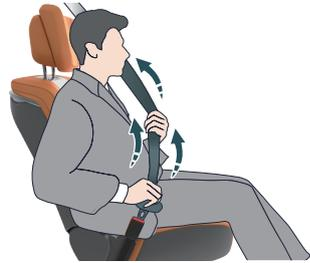
Front seat belts and rear seat belts on both sides seat are equipped with pre-tensioning and force limit devices, which can significantly improve the protection of occupants in the event of a forward, sideways or rearward collision. According to the impact intensity, after the pre-tensioning device is triggered, the seat belt can be tightened immediately, and the force limiting device can relieve the pressure of the seat belt on the passenger's chest and enhance the protection function.
