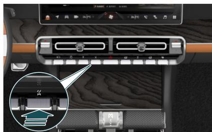
Press the front differential lock button to lock/unlock the front differential lock.
