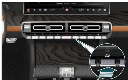
Press the crawl control button to turn on/off the crawl control function.
