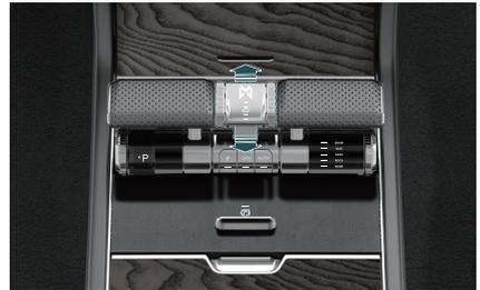
When the ASC system is in unlocked mode, you can operate the suspension adjustment handle to adjust the suspension up/down, and the vehicle height can be adjusted to five positions: "Economic height (Aero)", "Standard height (NRH)", "Off-road height (R1, R2)", and "Escape height (R3)".
