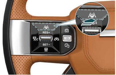
When the ICA is turned off, press the ICA button shown in the figure, the ICA function will be turned on with one attempt for activation.
