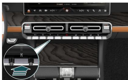
Press the rear differential lock button to lock/unlock the rear differential lock.
