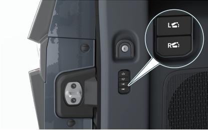
Press the "L"/"R" buttons on the left side of the trunk to fold/restore the rear seat backrest.
