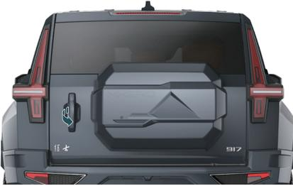
When the vehicle is locked, approach the vehicle identification area with the smart key and Bluetooth key and press the tailgate handle inside switch and pull outward to open the tailgate.
