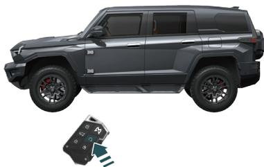
Press and hold the smart key START/STOP button
