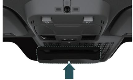
The vehicle is equipped with automatic anti-glare interior rearview mirrors. When driving at night, if there is strong light behind, the interior rearview mirror will automatically adjust the mirror reflectivity to reduce the reflection of the strong light.
