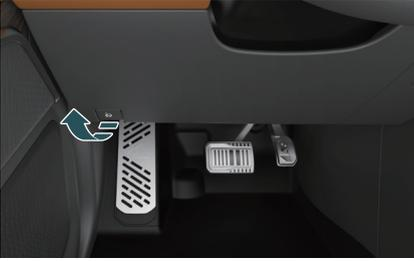
The engine hood opening handle is located on the lower left of the driver side instrument panel.
