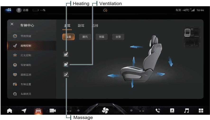
The front seats and both sides of the rear seats of the vehicle has heating, ventilation and message functions, which can be activated as needed to improve driving comfort.
