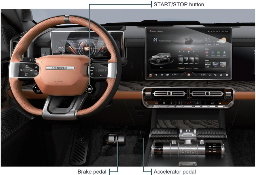
The vehicle is equipped with a START/STOP button. The START/STOP button can only be operated when the vehicle detects the smart key or Bluetooth key.
