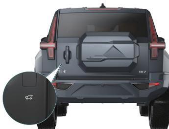
When the tailgate cannot be electrically opened, emergency opening of tailgate is allowed from the inside of the vehicle:
