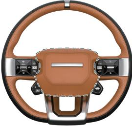
When the steering wheel is pressed in any position in the middle, the horn will sound, and when it is released, the sound will stop.
