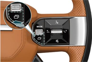
TPMS can monitor tire pressure and temperature in real time when the vehicle is running. After the START/STOP button is turned on, the display information of the instrument cluster can be switched by pressing the menu button
