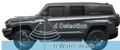
The wading induction system detects the height between the bottom of the left and right exterior rearview mirrors and the water surface through ultrasonic radar installed at the bottom of the mirrors. It calculates the current wading depth based on the real-time height of the vehicle, displays the current wading depth information on the CSD, and emits a warning sound to remind users when the vehicle has a large wading depth.
