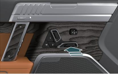
Press the leg support adjustment button forward and backward to adjust the position of the leg support forward and backward.
