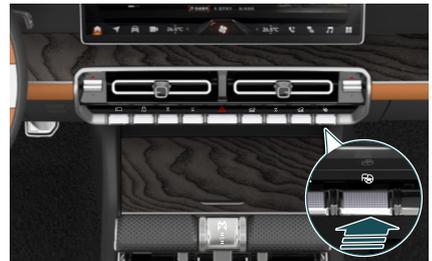
Press the APA button to activate the APA function. After activation, follow the graphics and text prompts displayed on the CSD to complete automatic parking.
