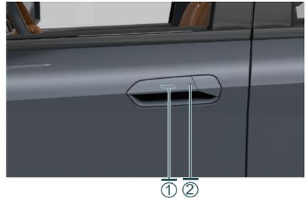
When the vehicle is in a locked state, carry the smart key or Bluetooth key, press the inner button ① of any door handle (as shown in the above figure), the vehicle will be unlocked, the left and right turn signal lamps will flash twice, and the exterior rearview mirrors will be unfolded automatically.
