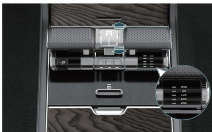
Toggle the all-terrain mode lever forward and backward to switch to all-terrain mode: Snow mode (SNOW) → Mud mode (MUD) → Sand mode (SAND) → Rock mode (ROCK) → Wade mode (WADE) → Snow mode (SNOW).
