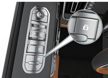
On the driver side, you can press the child safety lock button to activate the child safety lock function to prevent children from opening the car door from inside the car.
