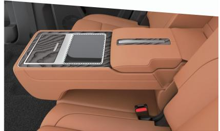
The rear seat armrest screen is located on the rear seat center armrest, and can be used by flipping the rear seat center armrest to the lowest position.
