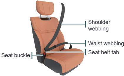
When the vehicle brakes in an emergency or collides, the seat belt can restrain the driver and occupant on the seat, preventing them from having a secondary collision with other components in the vehicle, and ensuring that the occupants can be effectively protected by the airbag.
