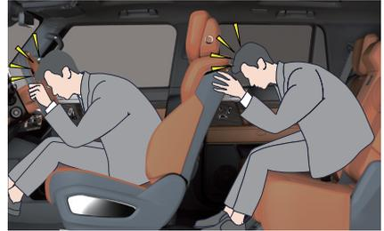
In the event of a vehicle collision, the driver and occupant who are not wearing seat belts may be thrown out of the vehicle and injured due to inertia. Even if the vehicle speed is very low, the force acting on human body during a collision is very large, and a secondary collision is very likely to occur.
