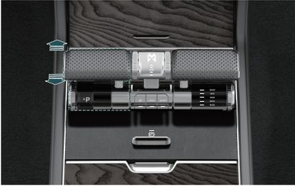
The vehicle has four gears: P, R, N, and D. After the vehicle is in the READY state, depress the brake pedal and push the shift lever back and forth to switch gears. The lower gear character block of the shift lever will turn to the transparent window area, and the corresponding gear will be displayed on the instrument cluster.
