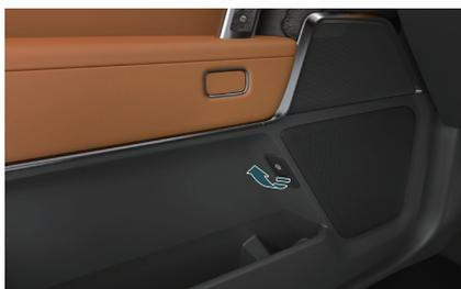
When the door cannot be opened using the electronic control internal door opening button, the emergency opening switch located above the door storage box can be pulled to open the door.
