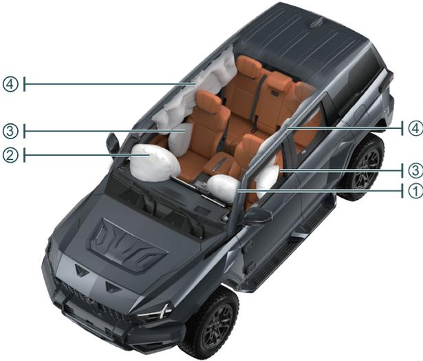
**① Driver airbag** (located under the steering wheel central cover plate)
