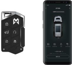
Press the smart key or Bluetooth key unlock button
