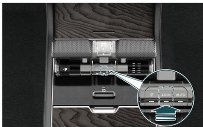
Press the suspension height locking button to lock the suspension height. In locking mode, the system will prohibit manual or automatic adjustment of suspension height.
