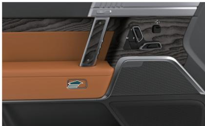
When the vehicle is stationary, press the electronic control internal door opening button to open the door at the corresponding side.
