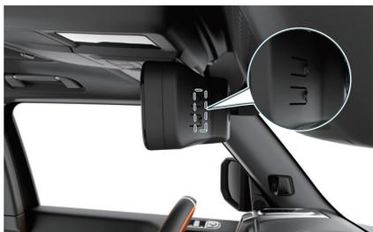
Press and release the mode switching button, select the up and down adjustment menu for the display area (camera shooting range), and press the "<" and ">" buttons to select the desired level.
