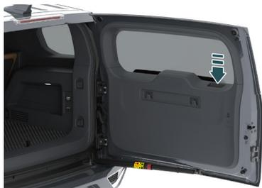
1. Check that the tailgate opening limiter is in the unlocked state;
