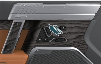
Press the side wing adjustment button up and down to adjust the angle between the side wings of the seat and the backrest.
