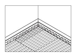
Align the profiles at the internal corners and press them into the joint.
