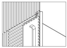
Apply joint to the places where the ceramics will be placed.
