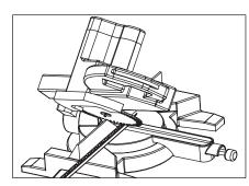
9 Cut profiles 45 degrees for internal corners.
