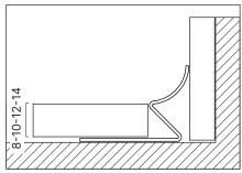
Pick the correct profile according to the tile thickness.
