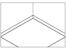
Place the tiles on the profile and make sure that their edges are fitted on the profile.
