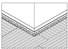
Align the profiles at the external corners and press them into the joint.
