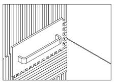
2 Apply joint and place the profiles anchor accordingly.
