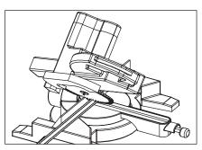
5 Cut profiles 45 degrees for internal corners.
