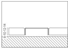
Pick the correct profile according to the tile thickness.
