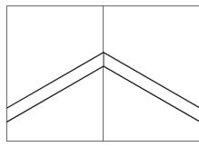
6 Place the profile between the tiles in internal corners. Make sure the profiles are aligned.
