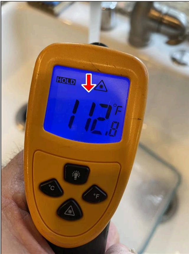
7.2 Item 1(Picture) hot water temp
