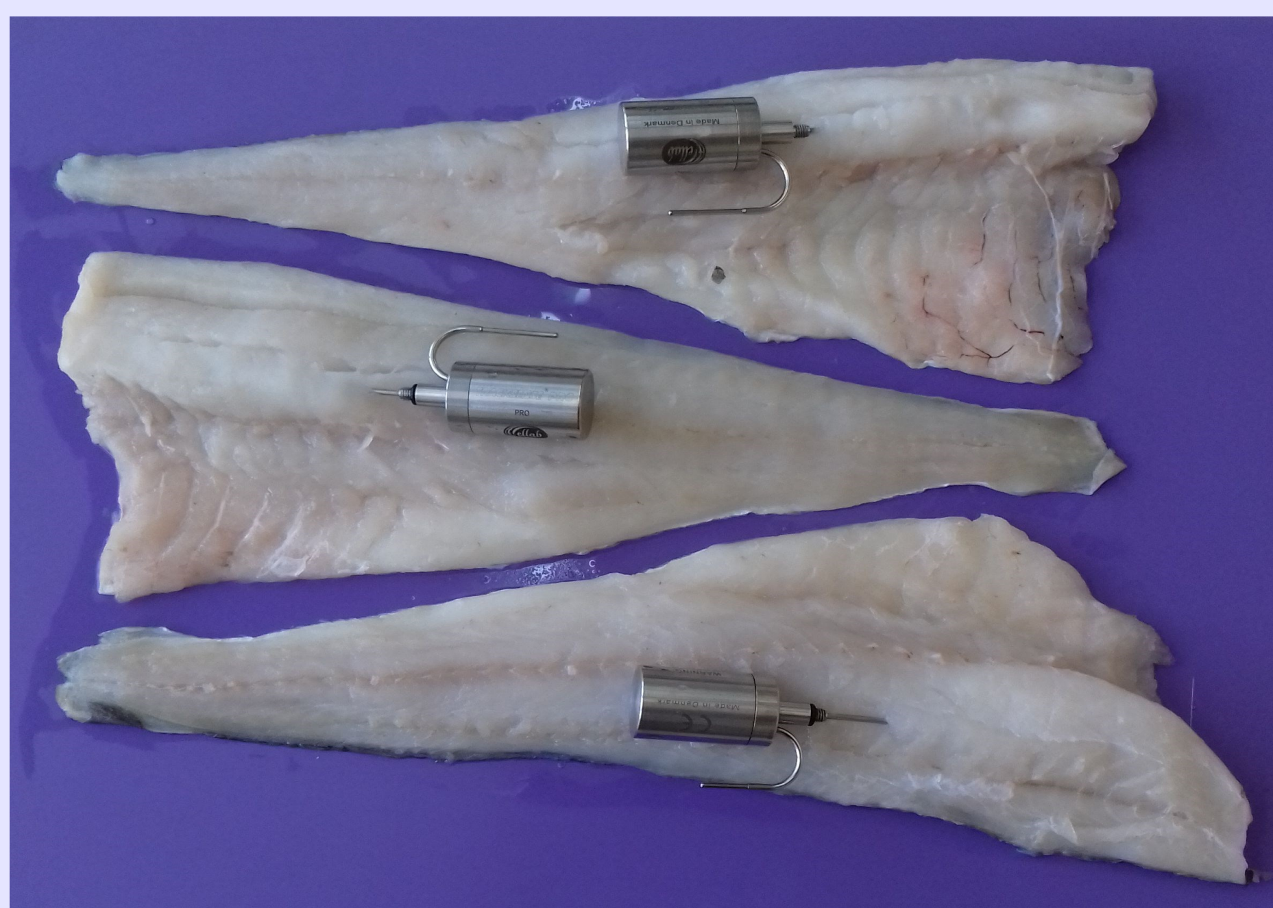
Photo 1. Cod fillets with thermocouples
